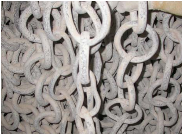
Figure 3. Thinned and warped round-link chain
