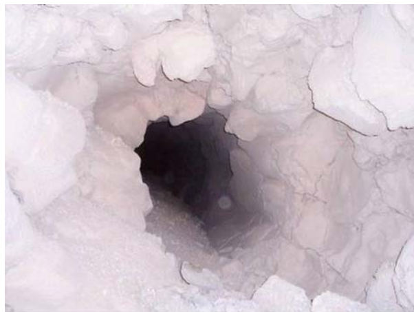
Figure 1. Ring formation in the PRPD lime kiln
