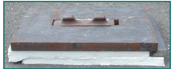
LINER PLATE AND BASED SHOWING FIBRE INSULATION
