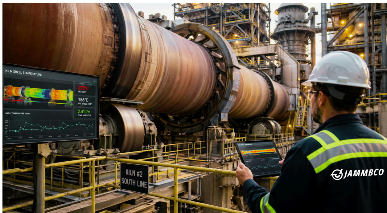
A wide industrial shot showing a rotary kiln, support stations, and an engineer reviewing shell temperature data.
